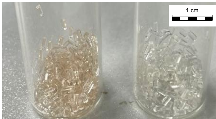
Figure 8 - Compound made from PLA with colourant (left) and pure PLA granules (right)
