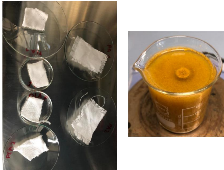
Figure – 9 Pre-washed PLA fabrics and Buriti dye solution
