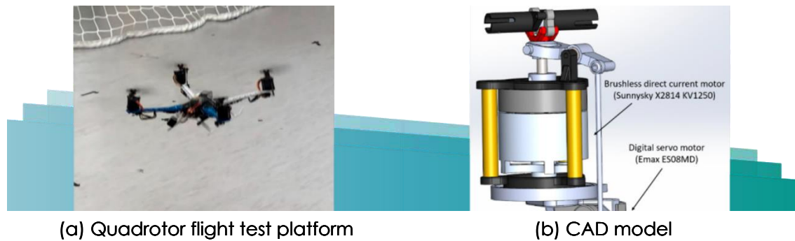
Figure 9 – VPP system implemented in a quadcopter
