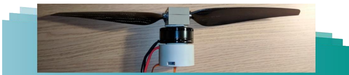
Figure 8 - Variable pitch propeller (16x6) with the engine
