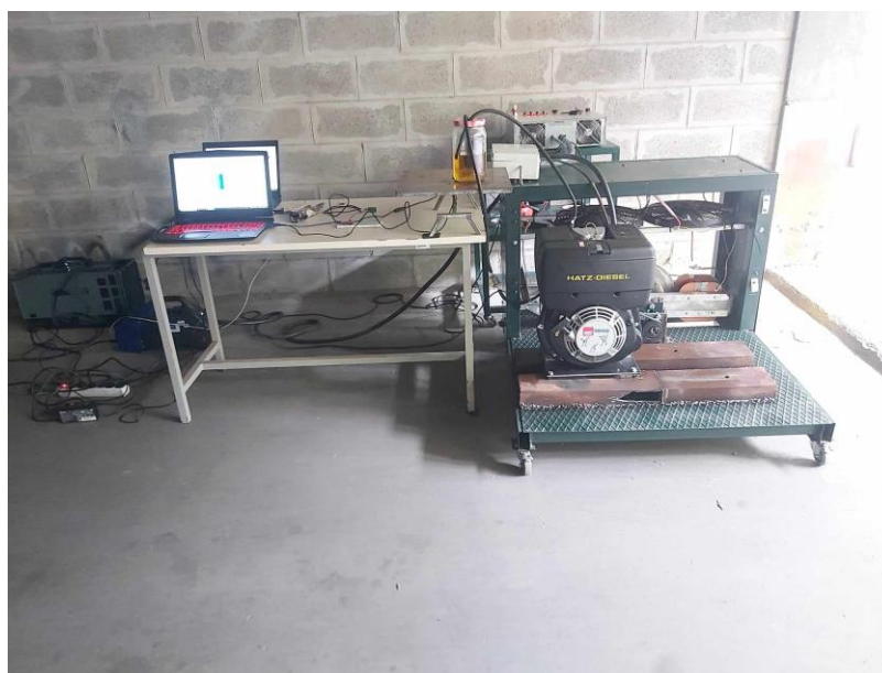
Figure 5 – Engine Bench-test Setup
