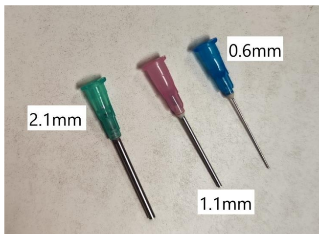
Figure 2 – Needles used with their respective external diameter
